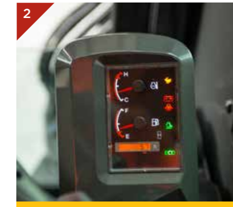
Easily visible monitor - includes travel speed, auto idle, eco mode, hour meter & engine management
