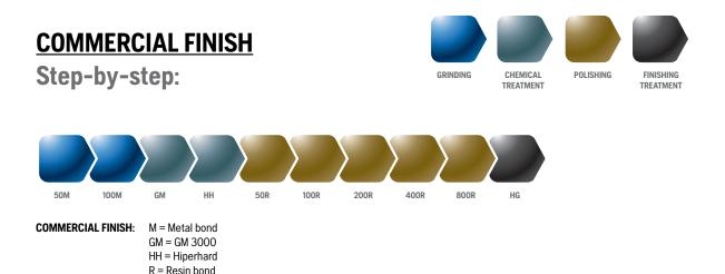
If the use of the P1242 50 grit resin bond tools is unsuccessful at removing excess Hiperhard (this would be the case if puddling Hiperhard is left to dry/cure on the surface), use T80 100 grit transition copper bond polishing pads in a semi-wet grinding fashion with water. Then move on to step 4 with P1243 100 grit resin bond floor-polishing pads.
