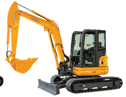
HD45V4 Operating Weight 4855kg Max Digging Force 31.0kN (3160kgf) Engine KUBOTA V2403-DI Options - Cabin or Rops Canopy - Steel or Rubber Tracks
