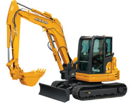
HD85V4 Operating Weight 8440kg Max Digging Force 55kN (5608kgf) Engine YANMAR 4TNV98C Options - Cabin or Rops Canopy - Steel or Rubber Tracks
