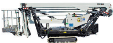
Model: 22.10 Weight 2980kg Working Height 21.7m
