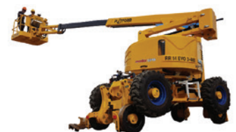
Model: RR14 EVO3 Rail Boom Weight 13400kg Working Height 14.4m
