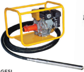
GE5L Flexible shafts 6m Head size 28, 38, 45 & 70mm Honda GX120 4hp
