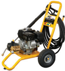
YR3000AR Pressure 2600psi Max flow 13.5 L/min Honda GX200 6.5hp
