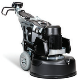
HTC DURATIQ 8 T8/RT8/X8/RX8 Power 12 / 15 kW Width 800mm Discs 270mm 3 or 4 disc Weight 499-574kg
