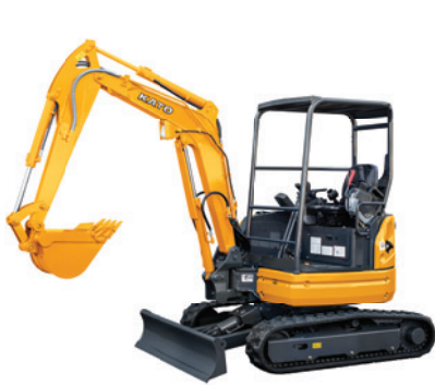
HD25V4 Operating Weight 2555kg Max Digging Force 19.6kN (2000kgf) Engine KUBOTA D1305 Options - Cabin or Rops Canopy
