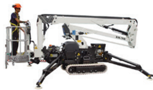
Model: 15.75 Weight 2060kg Working Height 15m
