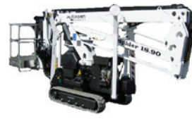
Model: 18.90 Weight 2457kg Working Height 17.6m
