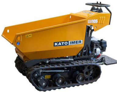
CARRY 105 Capacity 500KG Unit Weight 290 Kg Honda GX200 6.5Hp
