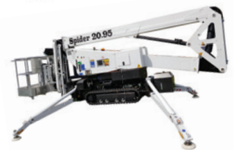
Model: 20.95 Weight 2800kg Working Height 19.4m
