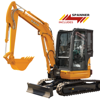
HD35V4 Operating Weight 3525kg Max Digging Force 29.1kN (2970kgf) Engine YANMAR 3TNV88 Options - Cabin or Rops Canopy - Steel or Rubber Tracks
