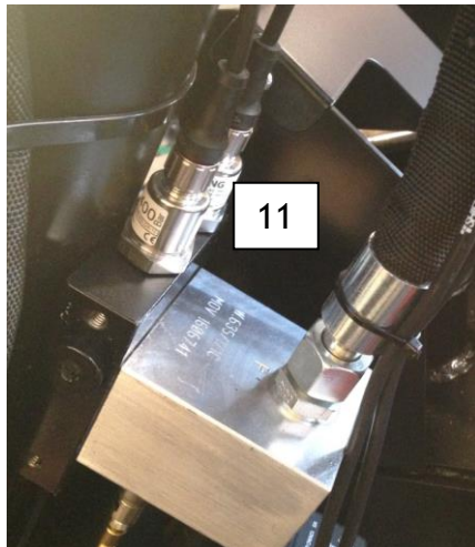
11. Pressure transducer for load control
