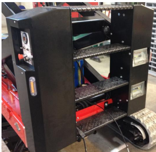
13. Ladder to access the platform
