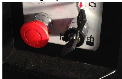
18. Ground control panel emergency button
