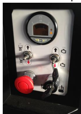
18. Ground control panel emergency button
