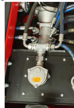
20. Oil tank refill cap
