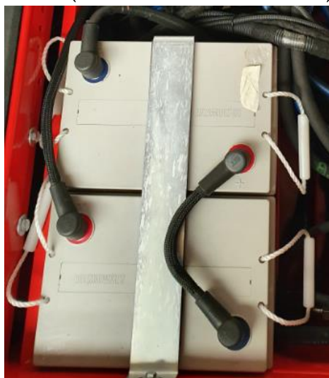
25. Batteries (ELC - BI-ENERGY Version)
