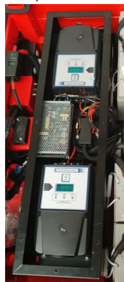
26. Battery charger (ELC - BI-ENERGY Version)
