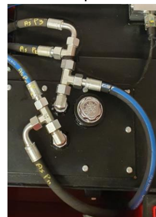
20. Oil tank refill cap
