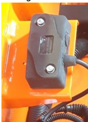
31. Chassis angle sensor
