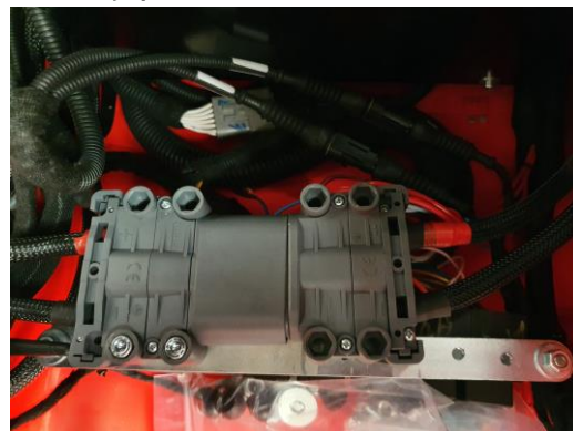
40. Battery power connector
