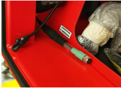
13. Remote control emergency cable connector
