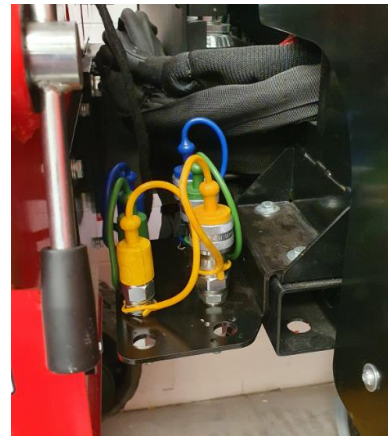
38. Valve kit crane (BI-ENERGY Version)
