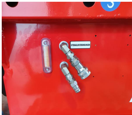
39. Hydraulic fast connector
