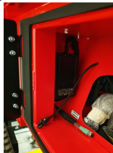
12. Remote control battery recharge compartment
