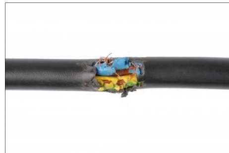
Damaged electric cable
