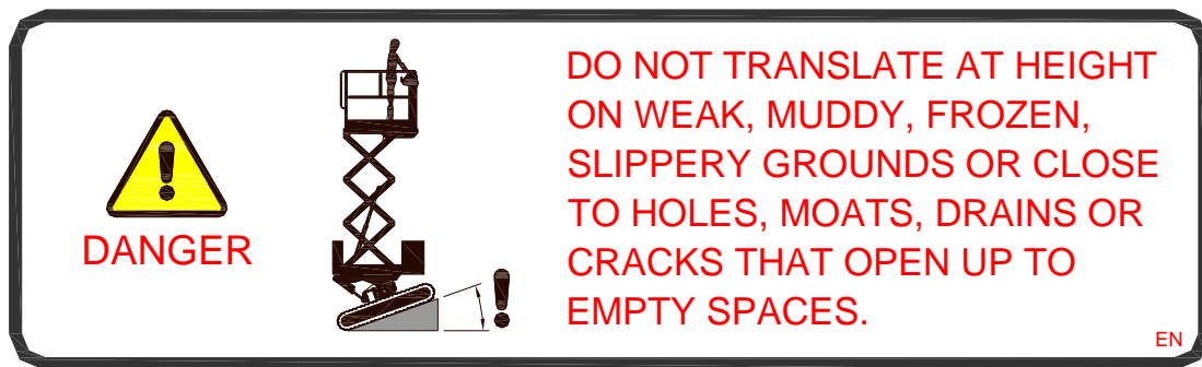
Plate with danger indication for inclined movement on slippery ground
