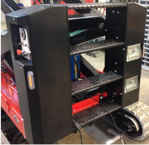
13. Ladder to access the platform
