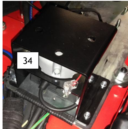
34. "Proactive levelling" limit switch
