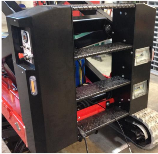
13. Ladder to access the platform
