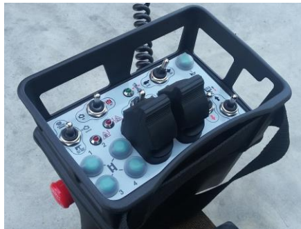
2. Control console emergency button
