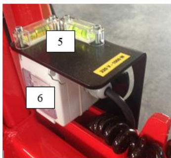
6. Socket on work platform
