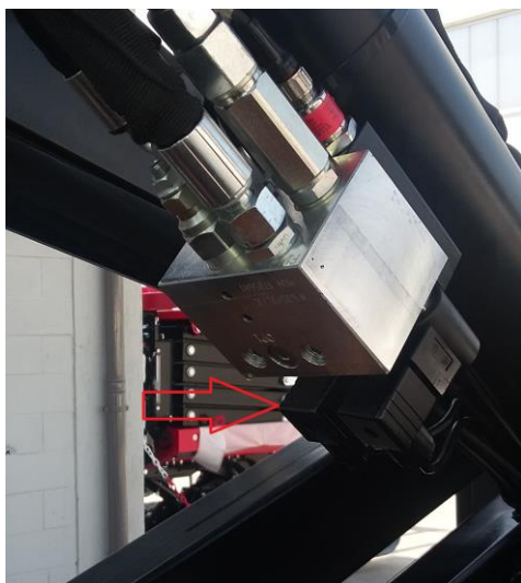
11. Seal solenoid valve on lower lifting cylinder SV18
