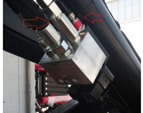
14. Pressure transducers to control the load in the basket
