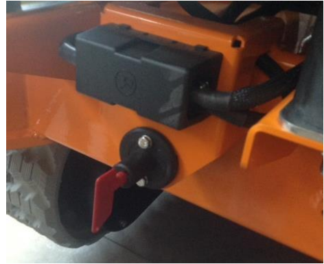
23. Battery disconnect switch
