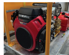
Engine: Honda IGX800 Electric start Pressure 3600psi Max flow 33 L/min
