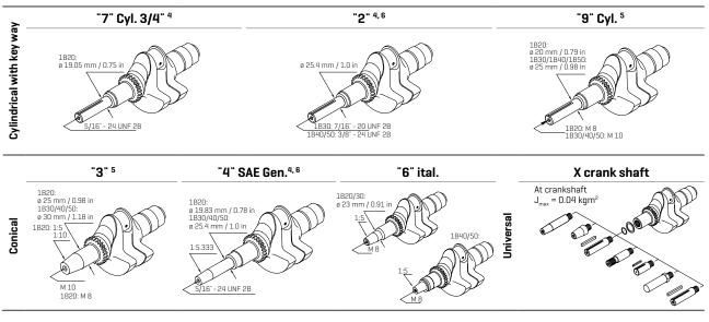
$<sup>^{\</sup>rm 4}$  According to SAE J 609  $^{\rm 5}$  According to LEMA LES 1203-1991  $^{\rm 6}$  Only for mechanically controlled engine types
