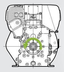
Power-take-off shaft, governor side, with max. engine speed, sense of rotation anti-clockwise.
