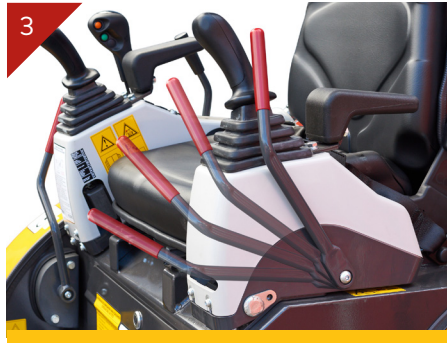
Gate Lock System Designed to lock all functions
