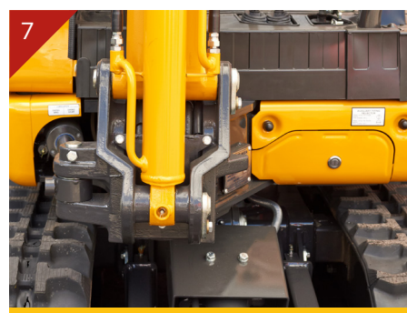
Offset boom - for increased visibility and boom rotation
