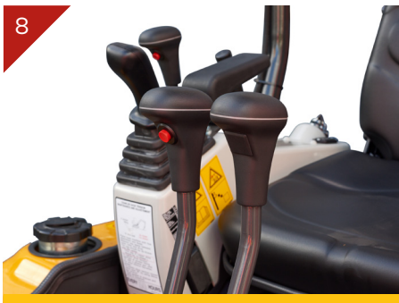
Two speed selection and track extension selection on control levers
