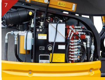
Large side cover for easy service access
