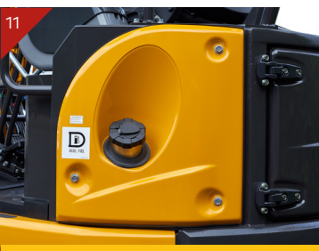
Fuel refill located in a convenient position
