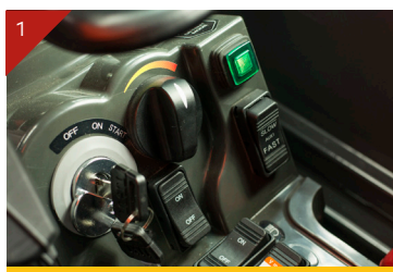
Centralised switches - includes key start, throttle dial, auto idle & eco mode
