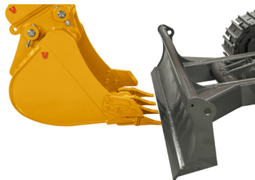
Close distance between Bucket Tooth and Dozer Blade
