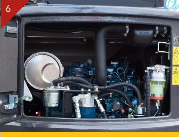
Large rear access for easy engine maintenance
