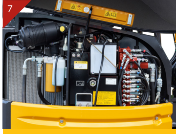
Large side cover for easy service access
