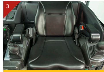
Full suspension seat - c/w retracting seat belt
