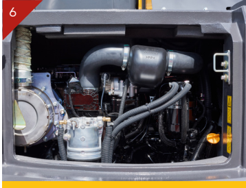
Large rear access for easy engine maintenance
