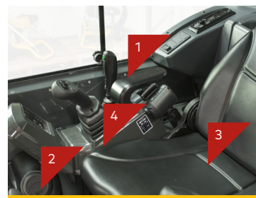
Full suspension seat - c/w retracting seat belt
