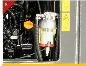
Water separator with indicator
