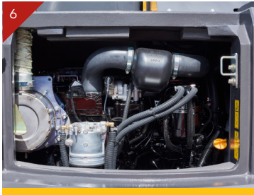
Large rear access for easy engine maintenance
