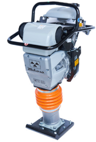
MTX85DY (Diesel) Weight 93kg Plate (mm) 340x285 Impact Force 15.7kN Honda GXR120 3.6hp
