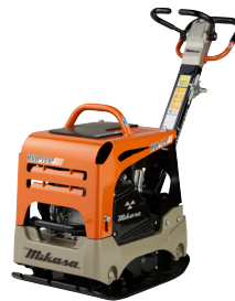
MVH128GH (Petrol) Weight 122kg Plate (mm) 590x400 Cent. force 23.5kN Honda GX160 5.0hp Start Recoil
