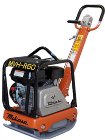
MVHR60H A (Petrol) Weight 68kg Plate (mm) 480x350 Cent. force 15.0kN Honda GX120 4hp Start Recoil *Comes with water tank
