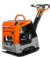
MVH208 Series (Petrol or Diesel) Weight 240kg Plate (mm) 720x500 Cent. force 37.0kN Hatz/Yanmar 6.7hp Start Electric/Recoil
