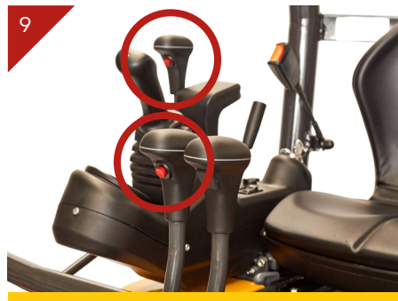
Two speed selection and track extension selection on joystick
