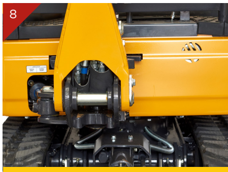
Offset boom - for increased visibility and boom rotation
