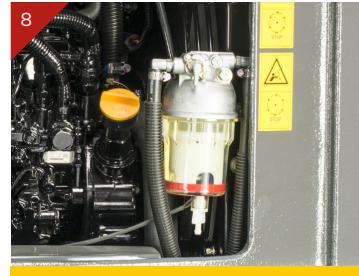
Water separator with indicator
