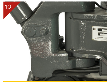
Single-structured Swing Pin
