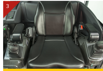
Full suspension seat - c/w retracting seat belt
