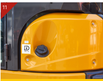
Fuel refill located in a convenient position
