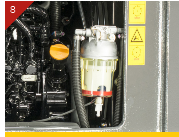
Water separator with indicator
