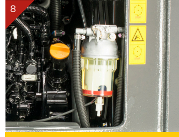
Water separator with indicator
