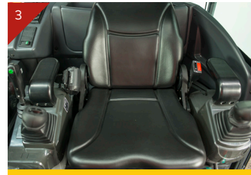
Full suspension seat - c/w retracting seat belt
