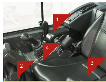
Full suspension seat - c/w retracting seat belt
