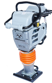
MTX70E (Petrol) Weight 75kg Plate (mm) 340x285 Impact force 14.9kN Honda GX100 3.0hp
