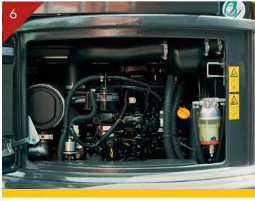
Large rear access for easy engine maintenance
