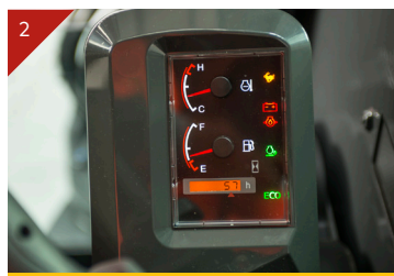
Easily visible monitor - includes travel speed, auto idle, eco mode, hour meter & engine management
