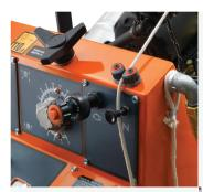
Clam cleat pointer rope holder Reduces pointer rope damage and holds front pointer at a set height.
