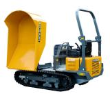
CARRY 110 Capacity: 1000 Kg Unit Weight: 830 Kg Yanmar Water Cooled 19.2 Hp
