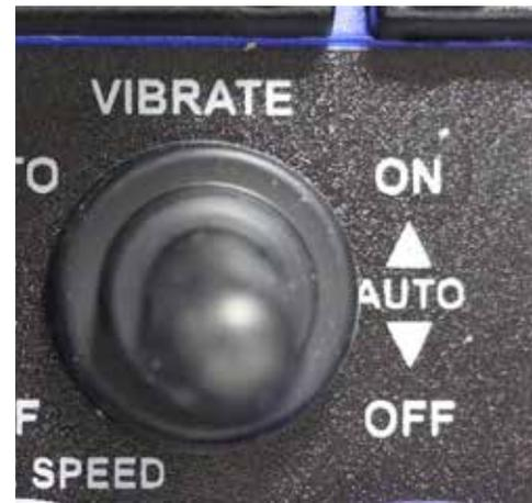
ON = Vibrator/Auger is turned on and stays on as long as the switch is in this position.
