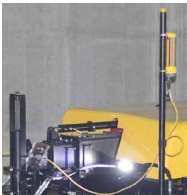
3. Attach the yellow laser eye cables to each device by aligning the grooves, then push the connector in and hand-tighten the screw ring to lock onto the eyes. Attach the other end of each laser-eye cable to the connectors above the screed head by aligning the grooves and then clamp the cam lock shut to lock the cables in place.
