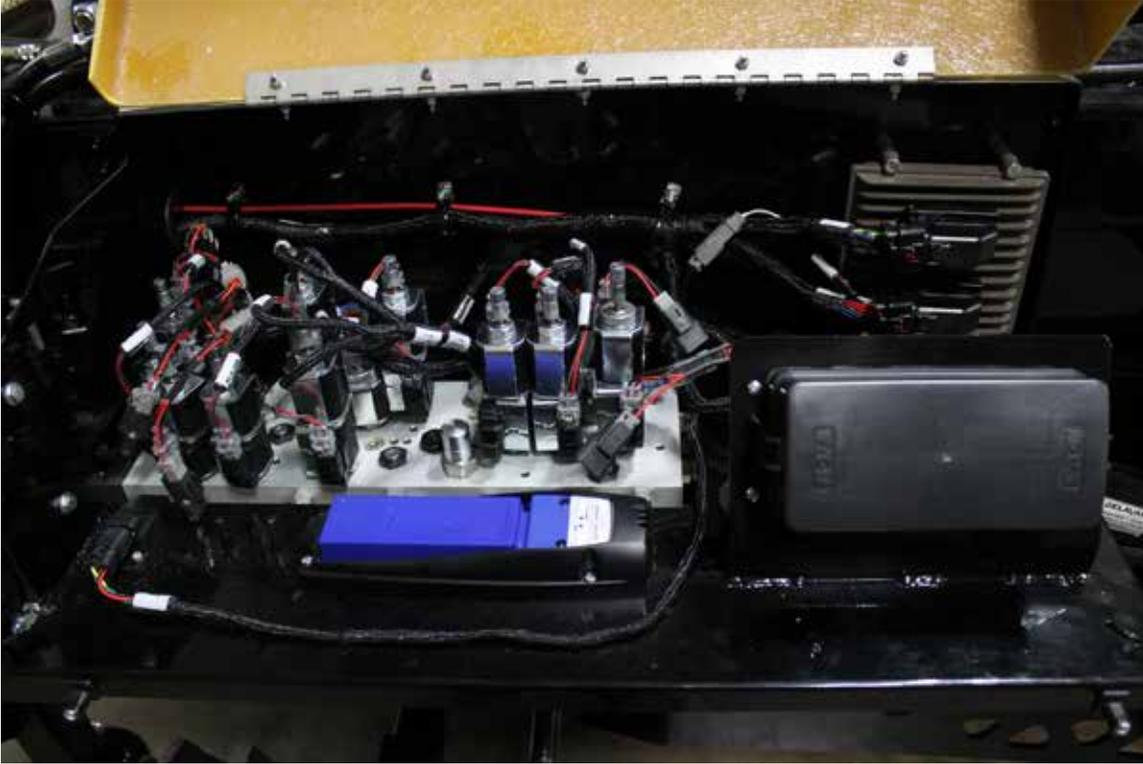
The SCREEDSAVER MAX PLUS has a state-of-the-art electronics system, and it's important to take care not to damage it. The electronics system on this machine is industrial grade, and gaskets have been placed at all wire junctions to minimize the impact of dust and moisture during normal use. For complete protection, all wiring routes are under the hood and through protective shrouds. **Under normal circumstances, no maintenance is necessary.**
