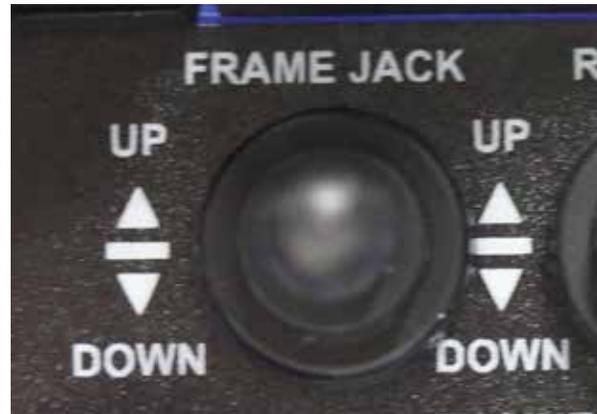
Note: The frame jack automatically raises the frame in **DRIVE** mode and lowers the frame in **SCREED** mode when the machine is placed into an automatic screeding/driving configuration. See the AUTO switch sections for more information.
