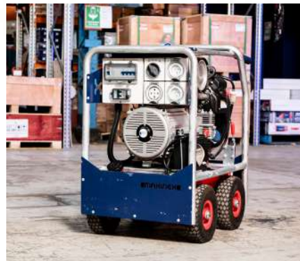
2. Power Generator 16 kVA
