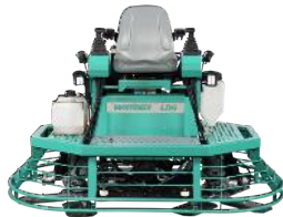
LD6 Hydrostatic Trowels Dual 6 Width 1905mm Diesel 23hp Weight 392kg
