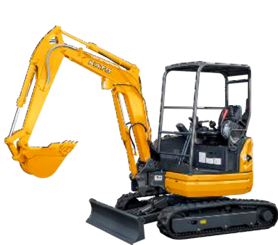
HD25V5 Operating Weight 2555kg Max Digging Force 19.6kN (2000kgf) Engine KUBOTA D1305 Options - Cabin or Rops Canopy
