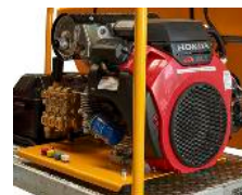
3. Engine: Honda GX390 Electric start Pressure 300psi Max flow 21L/min
