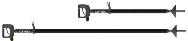
AIR-EX Excavating Tool Length (mm) 1180 - 2190 Effective 'cut' 100mm Compressor (cfm) 80-180
