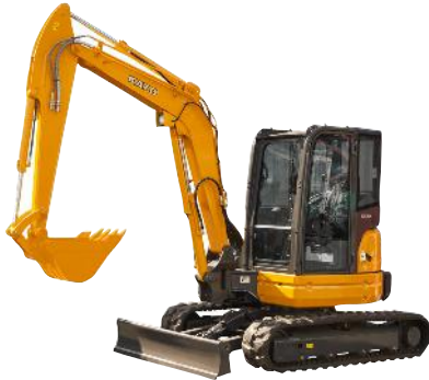
HD55V5 Operating Weight 5215kg Max Digging Force 31.0kN (3160kgf) Engine KUBOTA V2403-CR Options - Cabin or Rops Canopy - Steel or Rubber Tracks
