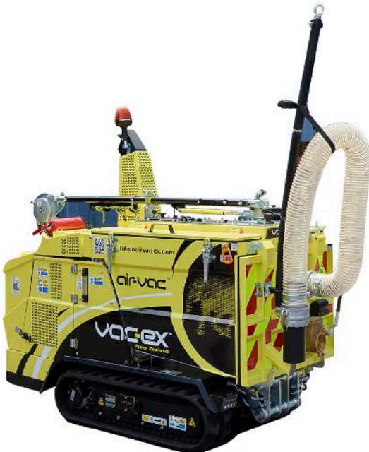
AIR-VAC Track Skip Capacity 0.2 m3 Unit Weight 1650kg Max Tipping 2540mm Hose inlet 125mm / 5"
