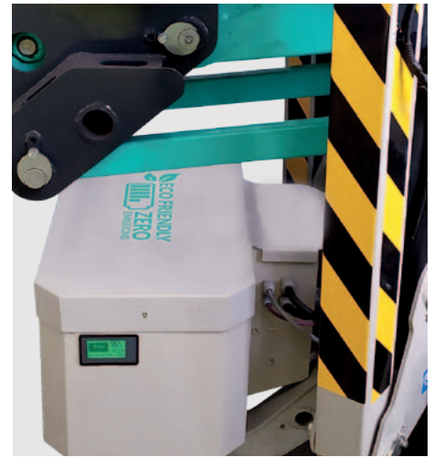
Lithium batteries compartment: protected and easily accessible for the charging cycle management. LCD display for charging status and remaining battery time.
