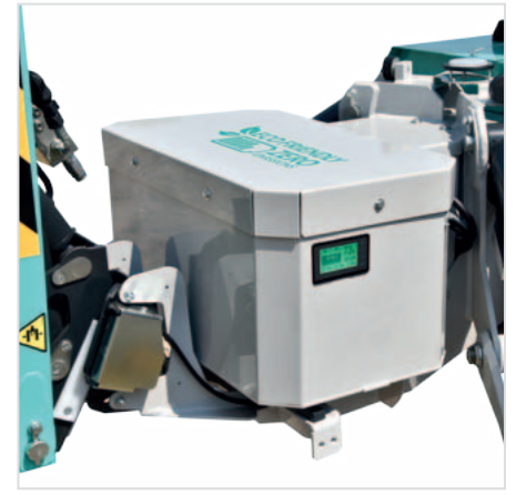
Lithium batteries compartment: protected and easily accessible for the charging cycle management. LCD display for charging status and remaining battery time.
