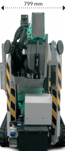
Compact dimensions for enhanced accessibility in any working site.
